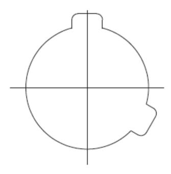
We can manufacture two or more keyways to produce a staggered cutting action when Gang Milling.
